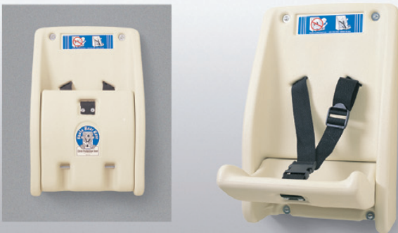
KB102-00 CHILD PROTECTION SEAT WALL-MOUNTED. Unit 12" W, 19" H (305 x 485 mm). Depth (closed) 5 3/4" (145 mm). Extension (open) 12 3/4" (310mm). Polyethylene, cream color.
