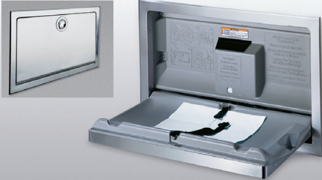
KB110-SSRE HORIZONTAL RECESSED STAINLESS FINISH. Unit 37" W, 23" H (940 x 585 mm). Depth (closed) 3/4" (20mm). Extension (open) 16" (405mm). Rough Wall Opening: 35 1/2" W x 20 1/2" H x 4" D (900 x 520 x 102mm).
