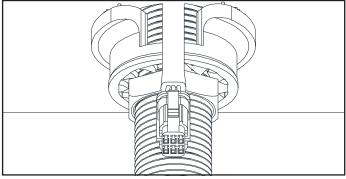
Sensor cable should not pass through plastic mounting washer.
