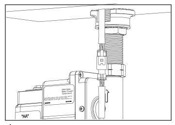
⚠ Do not engage the sensor for 30 seconds after the connection is made. The sensor will perform automatic calibration.
