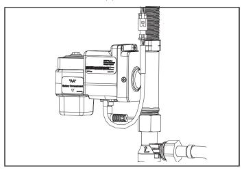
2.6. Connect solenoid cable from electronics module to sensor cable from spout.
