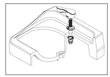
1.3. Ensure that slot in plastic washer is facing forward
