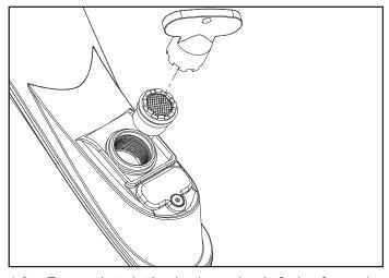
1.2. Install spout to sink using spout base gasket, plastic mounting washer, star washer and mounting nut (and cover plate for versions that are included).
