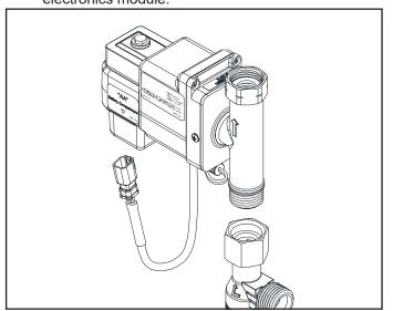
2.2. Open battery module using supplied Allen wrench and install supplied batteries in the electronics module
