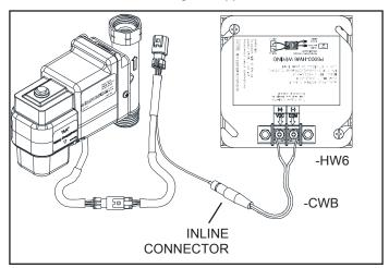
2.3. Tighten electronics module assembly to shank and connect water line(s).
