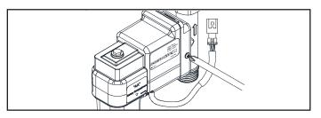
With screws removed, the electronics box can slide off and allow access to the solenoid for service
