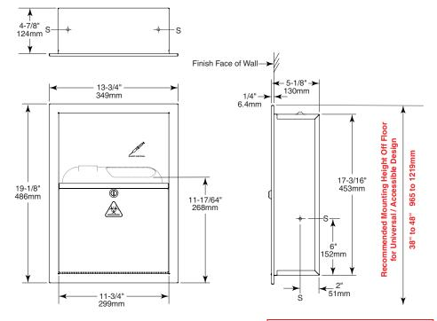
Rough Wall Opening 12" (305mm) wide 17-3/8" (441mm) high 5" (127mm) minimum recessed depth
