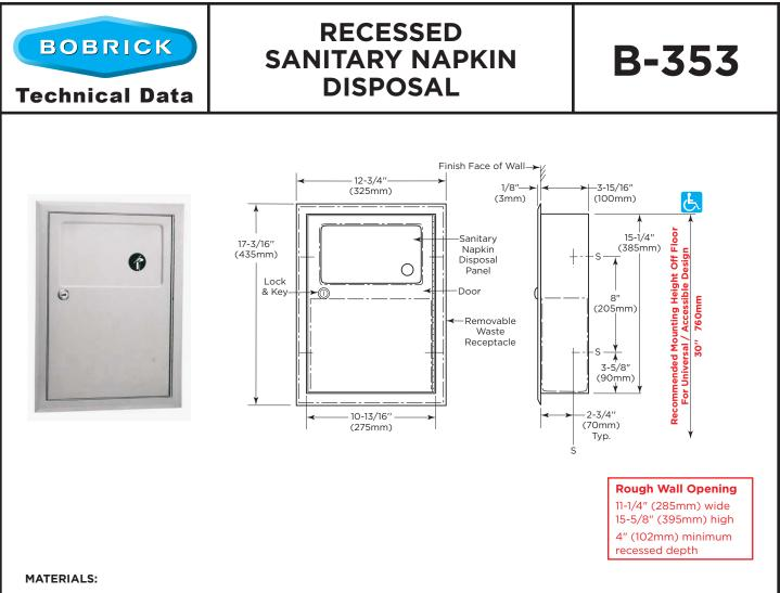
Cabinet - 118-8, type-304, heavy-gauge stainless steel. All-welded construction. Exposed surfaces have satin finish.
