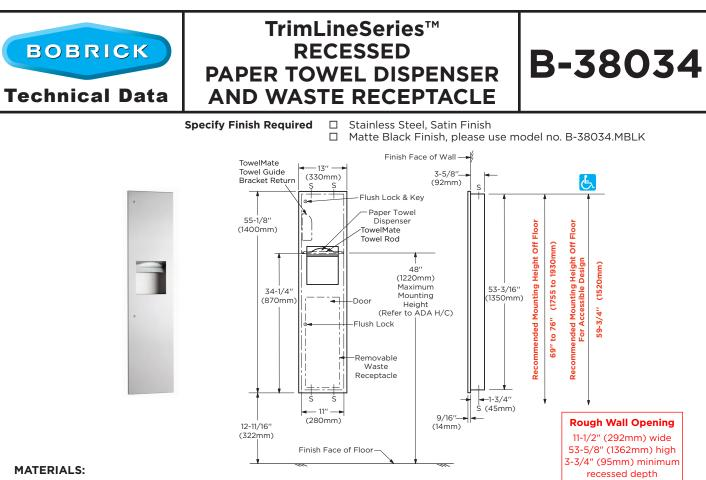
Cabinet - 18-8, Type-304, heavy-gauge stainless steel. All-welded construction.
