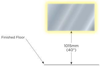
Please check installation height of the mirror with local barrier free guidelines. ADA (USA) requires that "Mirrors shall be mounted with the bottom edge of the reflecting surface no higher than 1015mm in (40") above the finished floor¹." For lit mirrors this means the dimension is to the inner most edge of the lit portion.
