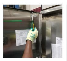
3b. When the pin is approximately <sup>3</sup>/<sub>4</sub> of the way into the hinge, make a slight bend to prevent the hinge pin from slipping out. Please refer to the <u>video</u> for an example.
