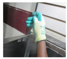
Reattach the metal chord (door check) by installing the hex nut that was removed in Step 1.
