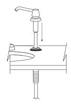
3. Secure the escutcheons by turning clockwise until lock snaps into position. Position Spout over the lavatory.
