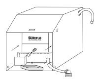
2. Screw Soap Supply Line Cap to Cartridge Outlet by turning clockwise. Soap should flow through the tubing.
