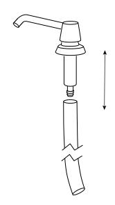
4. Insert soap pump assemblies with vertical tubes into Shanks.
