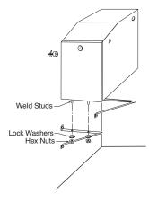
8. Place 2 lock washers and 2 hex nuts supplied on the weld studs on bottom of cabinet and tighten to secure cabinet to front bracket.
