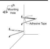
7. Without lowering the back of the cabinet. Place Cabinet on front Bracket aligning weld studs on bottom of cabinet through holes in front bracket and gently place back of cabinet on the back bracket which has the adhesive tape.
