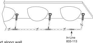
8. Screw Cable Supports into wall between each Soap Pump to support along wall.
