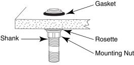
2. Insert soap pump assemblies with vertical tubes into Shanks.
