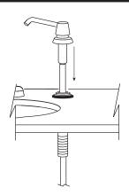
5. Secure the escutcheons by turning clockwise until lock snaps into position. Position Spout over the lavatory.
