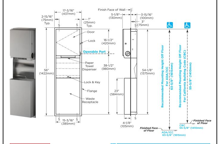
Rough Wall Opening 15-7/8" (403mm) wide 54-5/8" (1387mm) high 4" (100mm) minimum recessed depth
