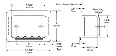
Rough Wall Opening 6" (150mm) wide 4" (102mm) high 4" (100mm) minimum recessed depth
