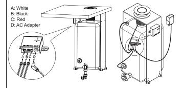
6. Ensure that the valve switches that are directly connected into the control boxes and reservoir tank are in the vertical (open) position.
