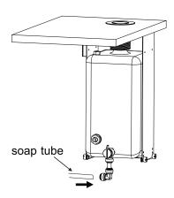
3. Connect a shut-off valve switch connector to the tubing at the end of the soap supply system. Make sure that the shut-off valve switch at the end of the multi-feed system is in the horizontal (closed) position. Reference image below currently shows in the vertical (open) position.
