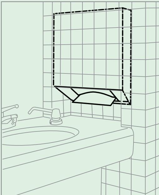
**Furred mirror installation** (figure 2) overhanging a bank of lavatories permits use of a full-depth vanity counter, a mirror brought conveniently close to the user, and towel dispensers above each bowl or between each pair. This arrangement also conforms to universal access codes which have height limitations that often prevent the conversational placement of both a mirror and recessed towel dispensers above the backsplash.
